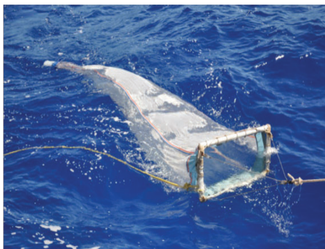
Figure 3. A Neuston Tow being conducted portside of the Seamans.
